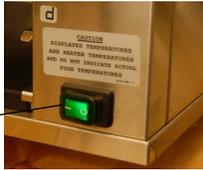
Allow 20 minutes for heaters to reach operating temperature. The button bar will read "WARM UP" as the unit warms up, they will display the product names.
