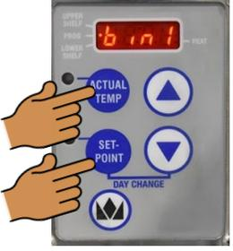
**2** To change a bin address, disconnect power to the unit and wait 10 seconds. Reconnect power to the unit and immediately press and hold the **ACTUAL TEMP** and **SETPOINT** buttons.
