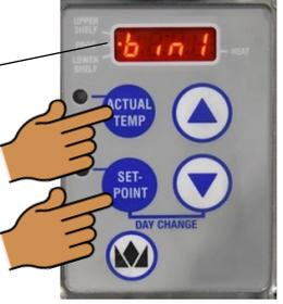
**3** Use the **UP** or **DOWN** Arrow button to scroll to the desired address. Press the **PRINCE CASTLE CROWN** button to store the new address.
