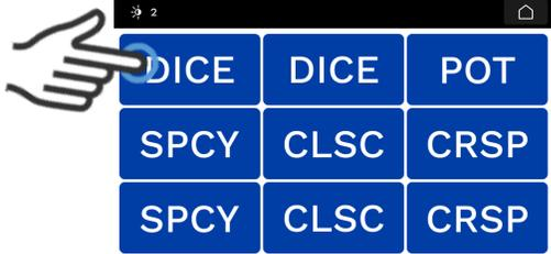
**7 Product FIFO System**—The unit utilizes a FIFO (First In, First Out) system to indicate to the user which pan to pull product from first when multiple pans of the same product are being held.
